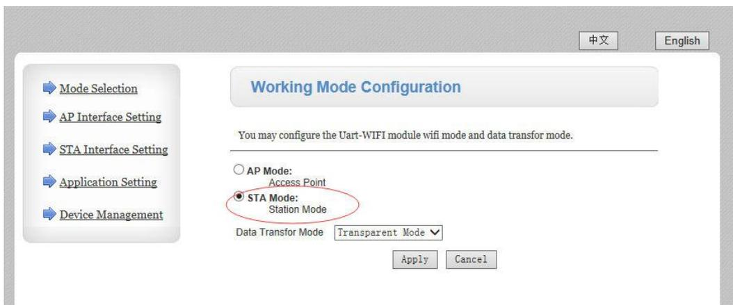
Remark: IP address in STA mode and AP mode could not be in same network segment.
